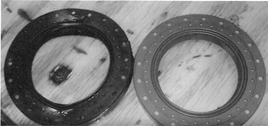
Figure 12: Old input shaft seal (left) vs. new input shaft seal (right).
